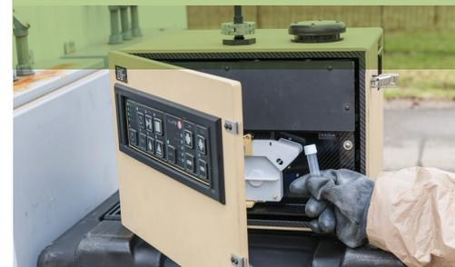
REBS also offers flexibility even after it has identified a pathogen. Its non-destructive analysis and automatic archiving capabilities support seamless integration into high-level biosurveillance operations for confirmatory, diagnostic and attribution analyses. This means that the samples it collects can be further analyzed to support attribution and medical diagnostic efforts.
